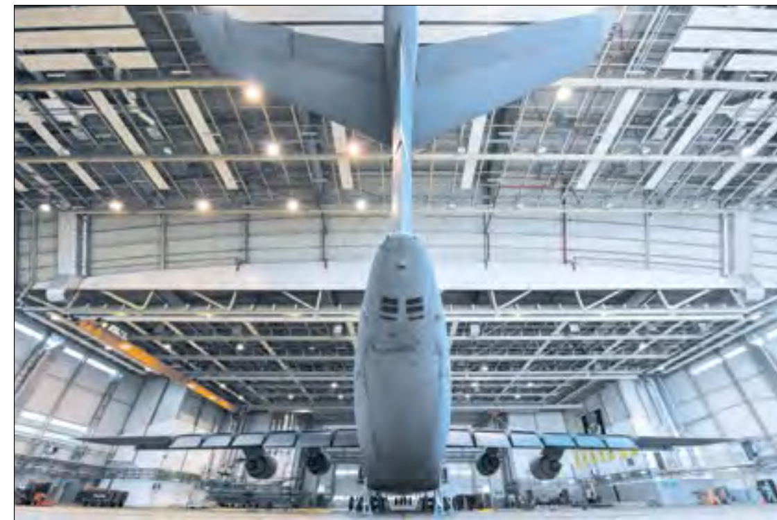
A C-5M Galaxy aircraft rests on six fuselage jacks for main landing gear repair May 3 at Ramstein Air Base, Germany. Flying out of Travis Air Force Base, Calif., to Ramstein, the aircraft's No. 4 main landing gear malfunctioned and the crew had to use the emergency backup system to make a safe landing. Airmen assigned to the 721st Aircraft Maintenance Squadron and 60th AMXS repaired it.
